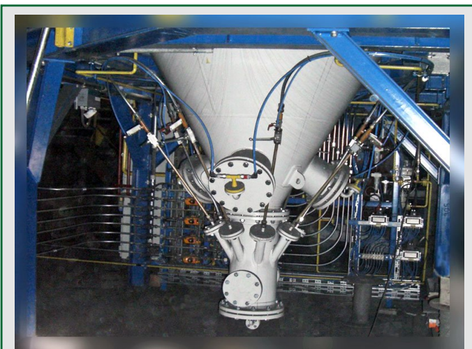
Bottom of a vessel distributor with single conveying pipelines
