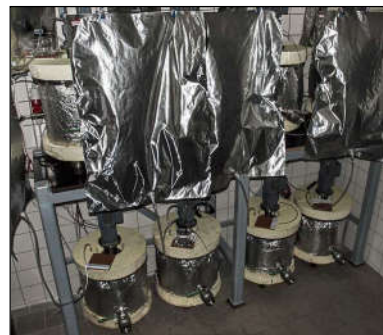
30 l-digester for batch-tests
