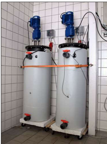
Continuous digester in the biogas laboratory
